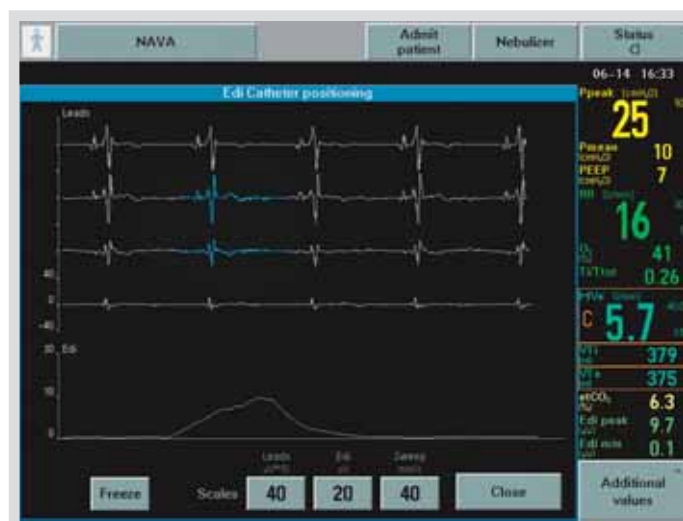
With the catheter properly positioned, a prominent P-wave should be visible in the uppermost channel with a continued decline of P-wave amplitude in the lower leads.
