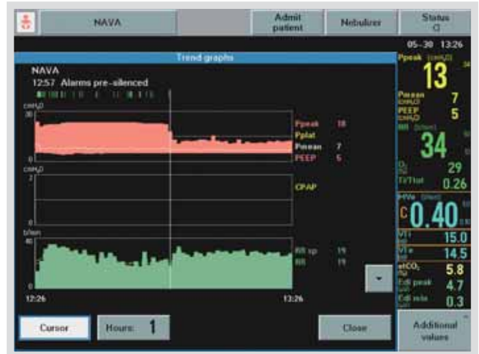
The decrease in pressure in this particular patient is clearly visible when switching from Pressure Support to Nava (shown in red). The green value shows respiratory rate.
