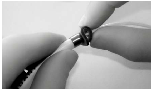
Figure D. Slide FLEXConnect™ Probe Fixation Device to metal tip of Probe.
